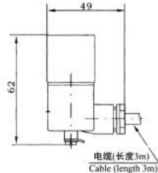
防爆线圈外形尺寸 Dimension of appearance of the anti-explode loop
